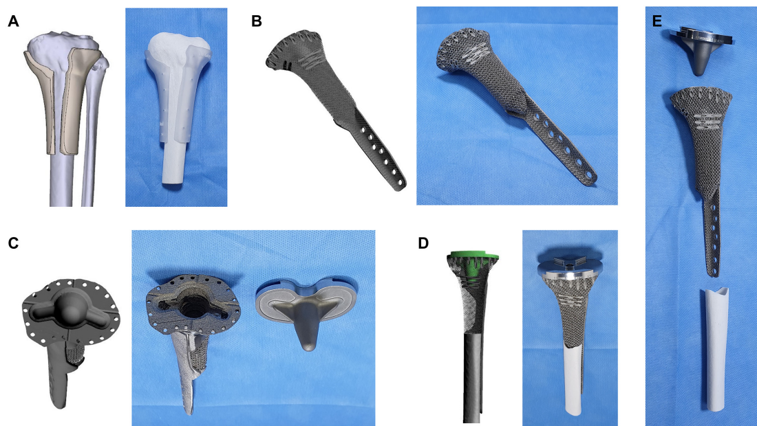
Fig. 4. Designs of the 3-dimensionally (3D)-printed products. Three-dimensional designs and photographs for the 3D-printed personalized surgical instrument (A) and the implant (B) are shown. (C) A design and photograph for the proximal tibial surface shows a matching socket for the tibial implant of conventional knee arthroplasty. (D, E) A design and photograph showing the 3D implant conjugated with the conventional knee arthroplasty implant.
